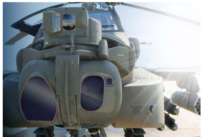
Figure 6 | M-DSA is an upgrade to the Apache's targeting and Modernized Target Acquisition Designation Sight/Pilot Night Vision Sensor (M-TADS/PNVS). Photo courtesy of Lockheed Martin.
