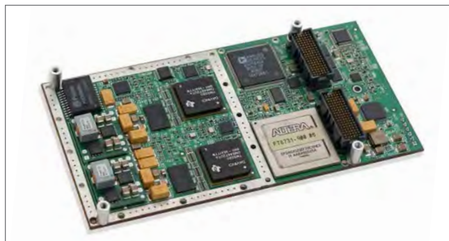
Figure 1 | The rugged ICS-8580 video compression XMC processes metadata as well as video.
