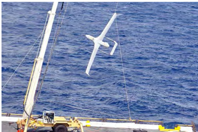
Figure 5 | A RQ-21A Blackjack UAS launching off the flight deck of a Navy vessel. Photo courtesy of Insitu.
