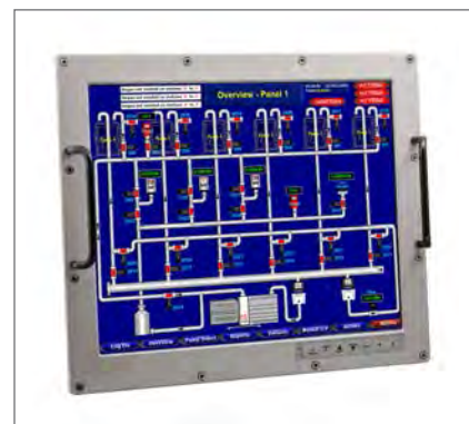
Figure 1 | Used in shipboard and military environments, the 19-inch SXGA (1,280 by 1,024) rugged display is sealed against liquid penetration and can be used below-decks as well. Photo courtesy of IEE.
